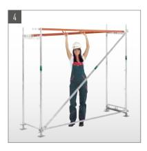
Mount decks, align perpendicularly to guard rail and frame with water level.
